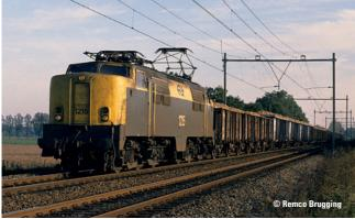
**Prototype**: Two type Eanos gondolas used on NS Cargo. Loaded with sugar beets.
