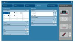
The window "Functions" has two (2) columns. The left column shows function activators; the right one shows the possible functions. Functions are already assigned to function buttons F0-F2 & F4. The previously set up running sound is immediately and correctly assigned here and needs no further editing.
