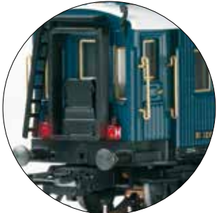
The red marker lights can be controlled digitally
